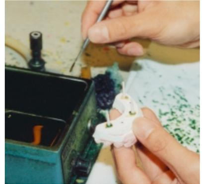
After the pins are glued with the Z-20 Spacer, a small amount of wax is added to prevent sticking to the base.
