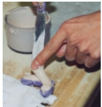
Before the initial set the refractory will thicken allowing it to be stacked.
